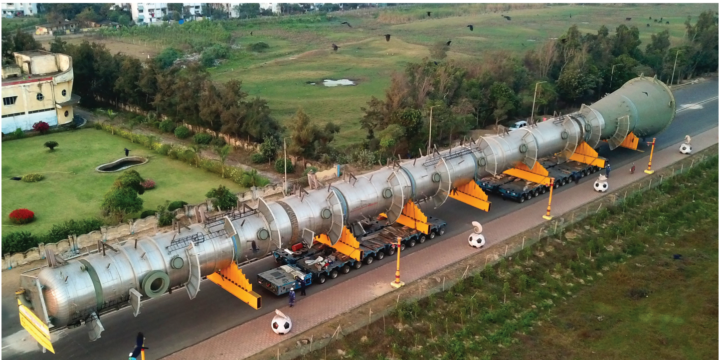
Wash Tower: 1155 MTs, 96.00 M (L) X 7.80 M (W) X 8.60 M (H) across multiple modes and vessels. This delicate giant made its way from a jetty on the west coast of India over axles, barges, heavy lift vessels and back onto axles onwards to a refinery on the east.
